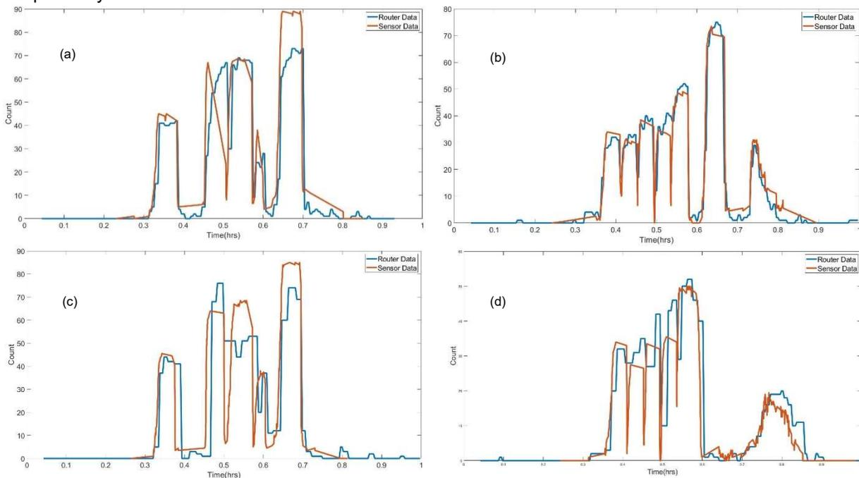
Figure 4: Sensor (C100) Occupancy count and Wi-fi Router Count vs time (a) Jan 22, 2019, (b) Jan 23, 2019, (c) Jan 24, 2019, (d) Jan 25, 2019
