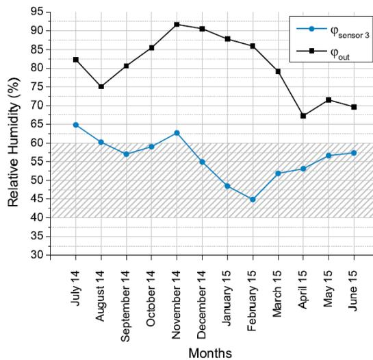
Figure 4: Self-regulation of moisture humidity in indoor environment (Soudani 2016)
