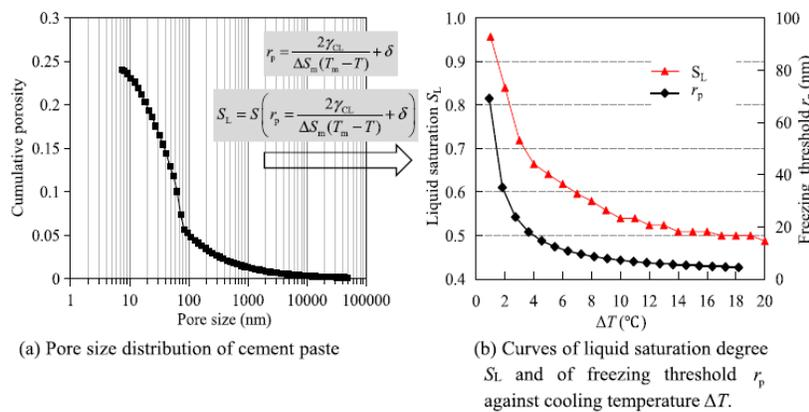
Figure 9: Calculation of the liquid degree saturation from pore size distribution during freezing (Liu, Qin and Wang 2018)
