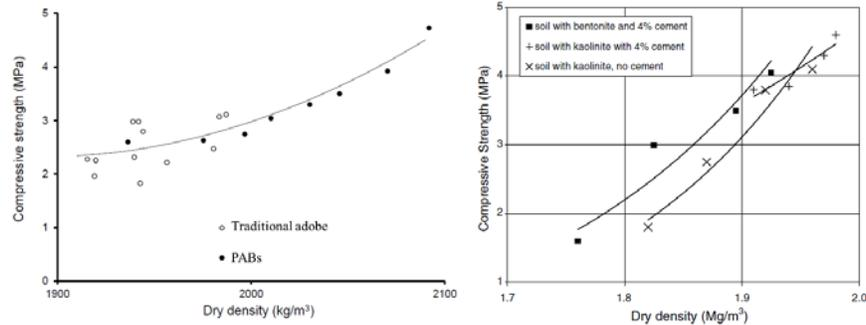
Figure 5: Evolution of compressive strength as a function of dry density (Champiré 2017)
