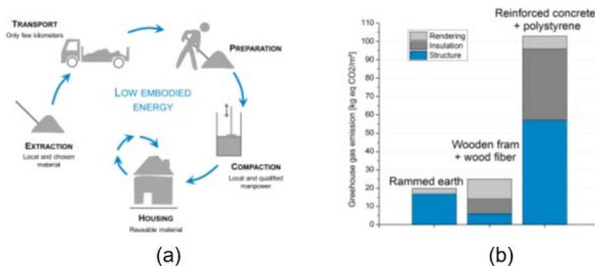
Figure2: (a) embodied energy during earth construction – (b) comparison of greenhouse gas emissions (Soudani 2016)
