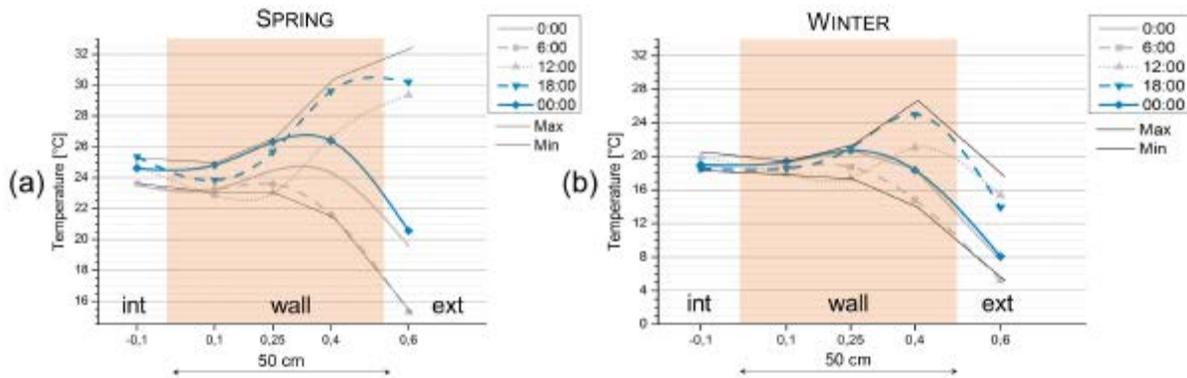
Figure 3 : Thermal comfort zone provides by raw earth heating inertia (Soudani 2016)
